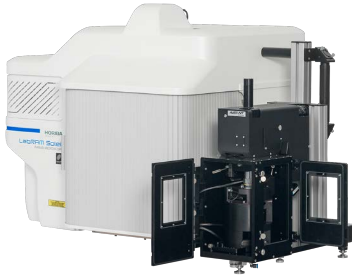
Figure: LabRAM Soleil Nano equipped with the environmental chamber*
