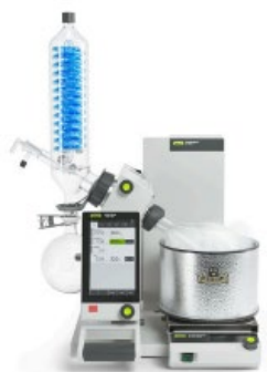
Figure 18: Shell (rotational) freezing using a Rotavapor® R-300 and the Dewar accessory (left). Sublimation in g/flask with (red square) and without (blue dots) rotational freezing (right).
