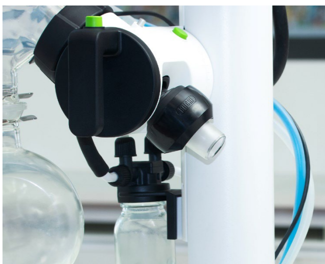
Figure 2: Combi-Clip for easy flask handling.
