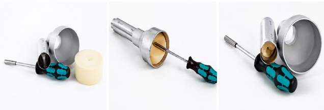
Figure 4: Putting the PUF filter into a SpeedExtractor E-914 extraction cell using a dedicated funnel.
